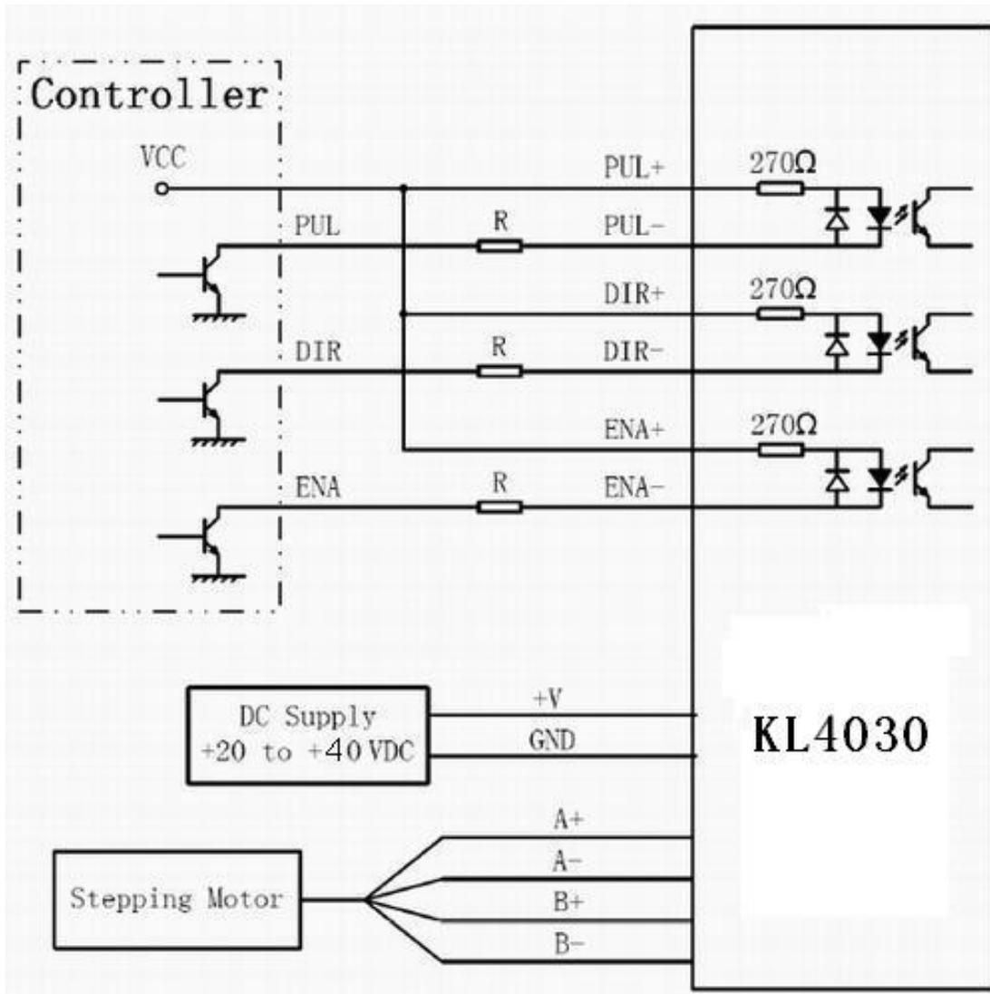
Figure 2: Typical Connections
